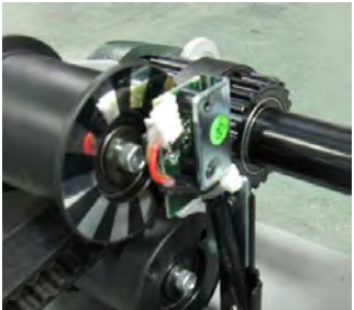
Inspect the optic sensor and the CLK indicator on the drive board.
